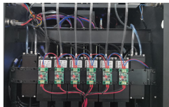
Ink Cartridge Heating System Provide guarantee for stable ink flow and color consistency no matter the temperature in the room
