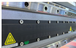
Magnetic Linear Motor and Metal Encoder Strip Ensure smooth and precise horizontal movement of the carriage
